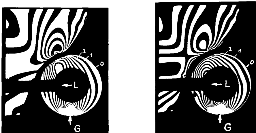
Fig. 31. Subluxated "hip joint". a. Slightly tightened "ligament". — b. Strongly tightened "ligament".
