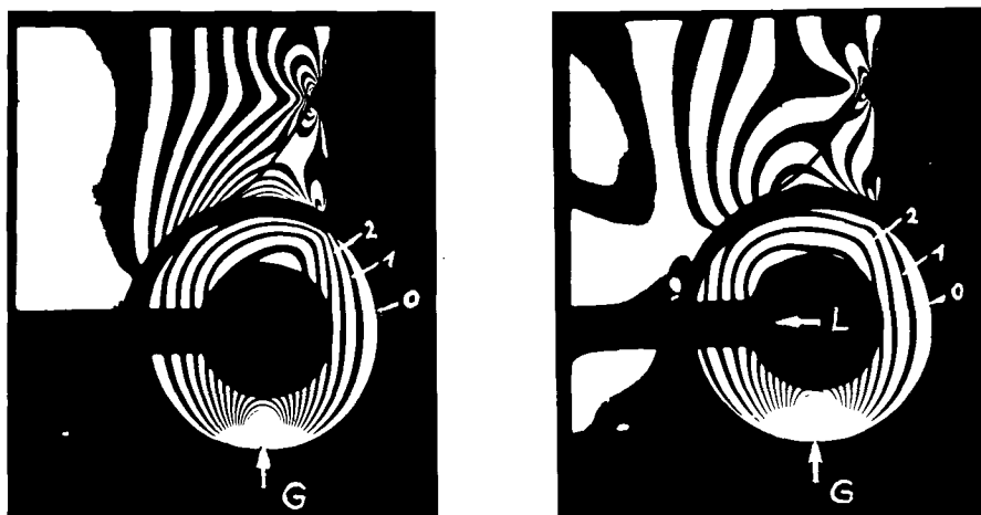
Fig. 34. Shelf at the level of the roof. a. The "ligament" is not tightened. — b. The "ligament" is tightened.
