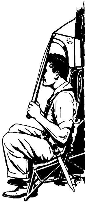
Fig. 33. Flyer in the shield-type of seat. This seat accelerates along a fixed track and is used for training and research purposes.
