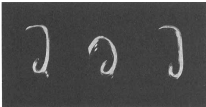
Fig. 17. Gruca hooks that failed are shown on right and left with a regular hook in the center for comparison.
