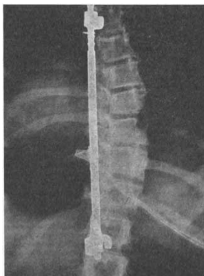
Fig. 28. Roentgenogram of distraction rod (Zimmer No. 1250) with strain gages applied in situ. (Patient 1).
