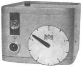
Fig. 26. The synchronizing clock allowing a film frame to be connected to a certain point on the recorded curves.
