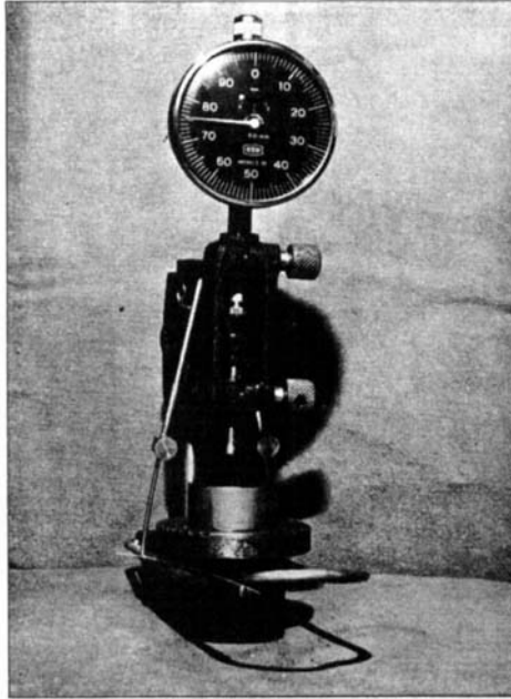
Figure 1. Micrometer used for thickness measurements.
