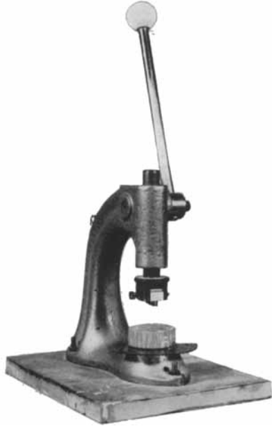
Figure 6. The modified press with a cutting die mounted.
