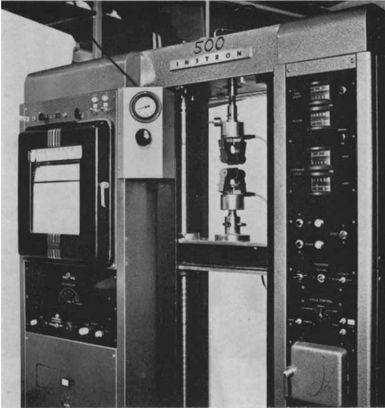
Figure 10. A detail of the Instron floor model tensile tester. The recorder is at the left, the control panel at the right. The air compression clamps and jaws faces are mounted.
