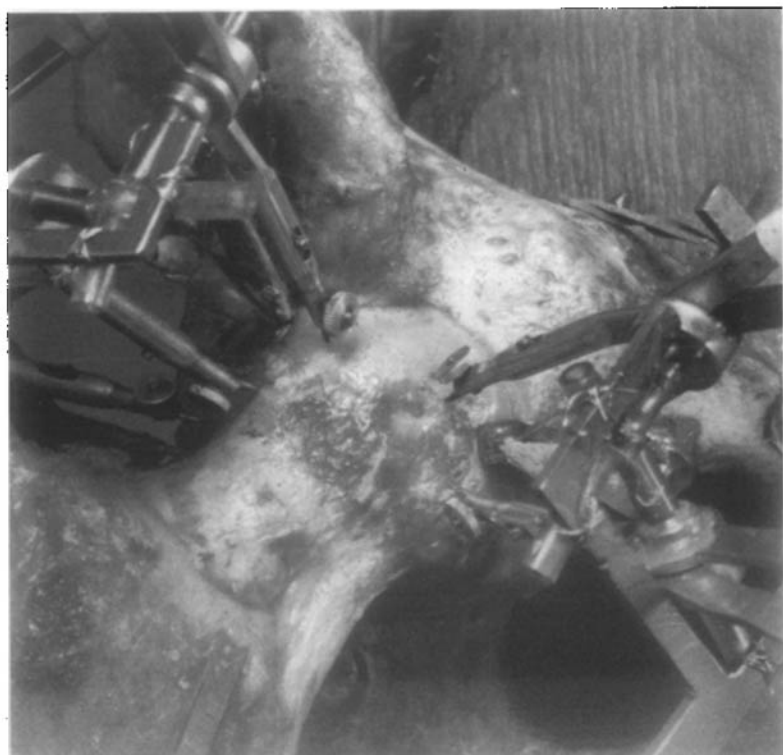
Fig. 9. Detail of calipers contacting the caput and measuring points of the acetabulum.
