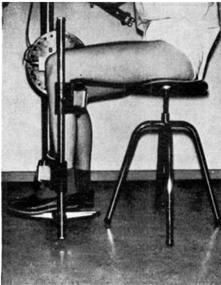
Figure 2. Measurement of strength of knee extensors, left leg. Healthy subject.
