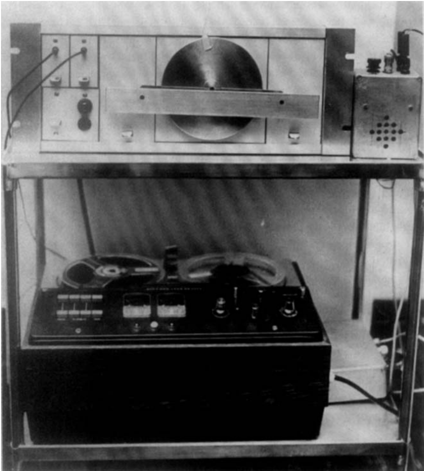
Fig. 4. The electro-mechanical apparatus with its frame and fly-wheel as the test subject will experience the system during the course of examination. Below a tape recorder and the standard programme.
