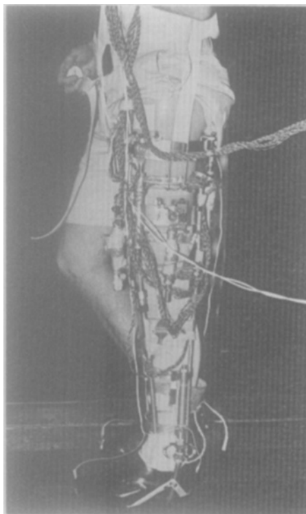
Figure 28. Lateral view. Author in the brace during mid stance phase. Note foot-switch circuit wiring attached to the shoes.
