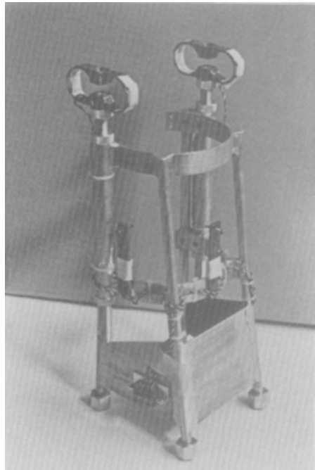
Figure 7. Lower segment upside down showing the ankle transducers, calf band beam transducers and couplings for attachment to the upper segment.
