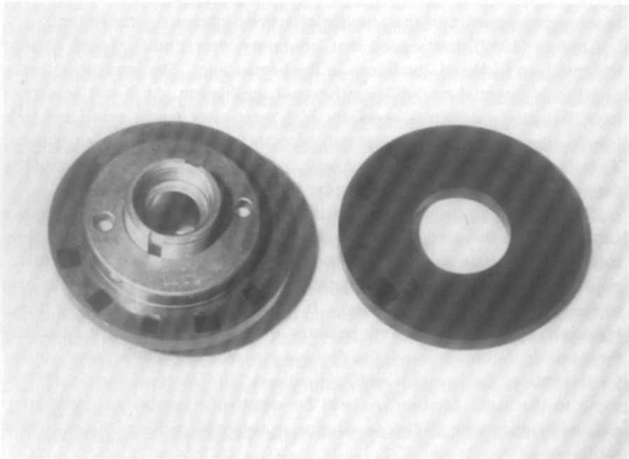
Figure 1. A specimen mounted on a collet and an unmounted specimen showing the characteristic "wear spots".
