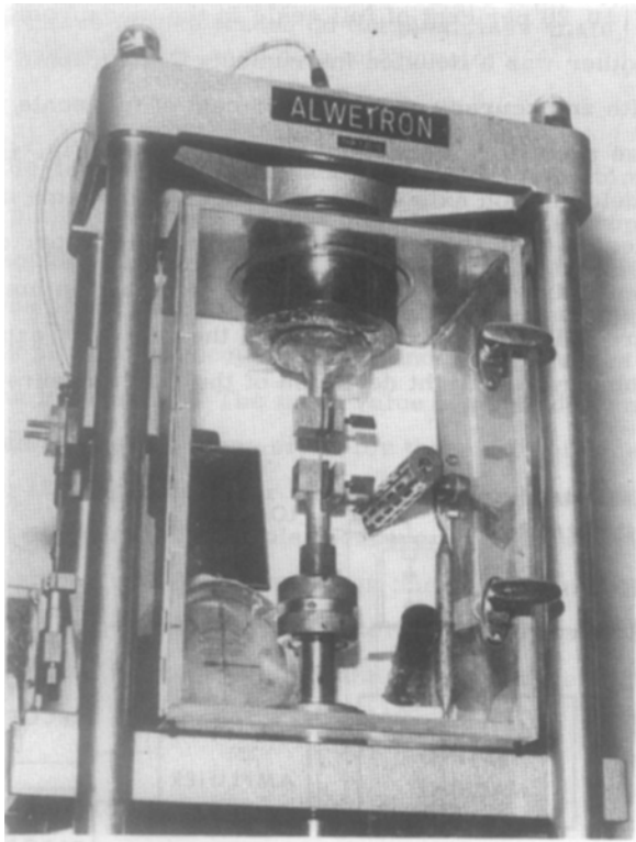
Fig. 5. Close up view of the Alwetron materials testing machine with the humidity chamber surrounding the test clamps. A tendon specimen is fitted between the clamps.
