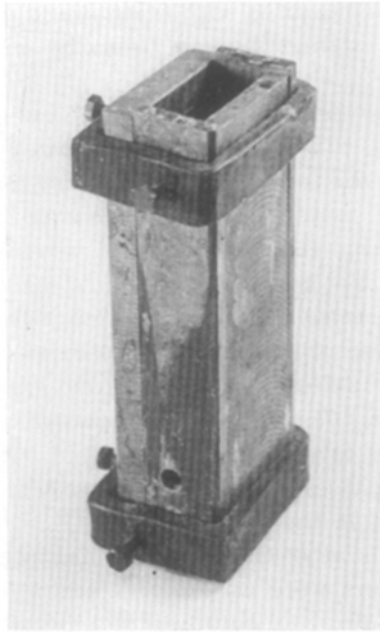
Figure 2. A photograph of the mould used for imbedding the ribs in acrylic resin. The walls are made of steel and they are demountable.
