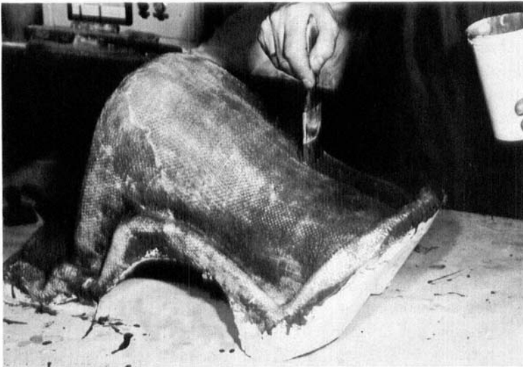
Figure 4. Lamination of the shell.
