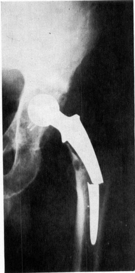
Figure 3. X-ray film 19 months postoperatively reveals the fracture in the middle third of the stem and angulation of the fragments.
