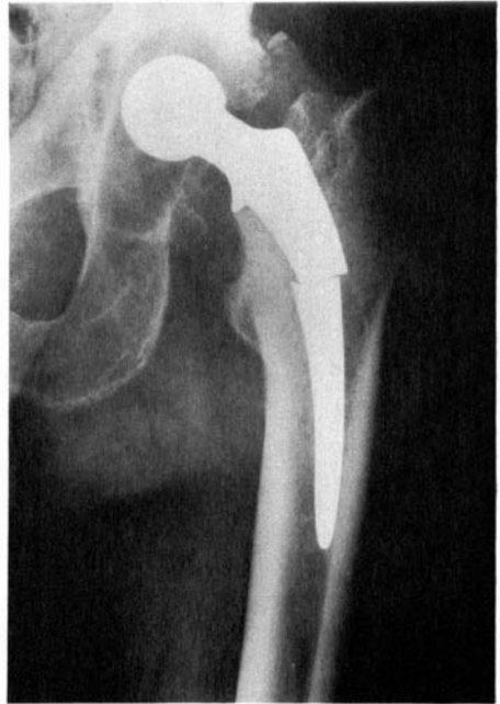
Figure 1. X-ray check 20 months postoperatively. Failure of the stem at the limit of the upper and middle third.
