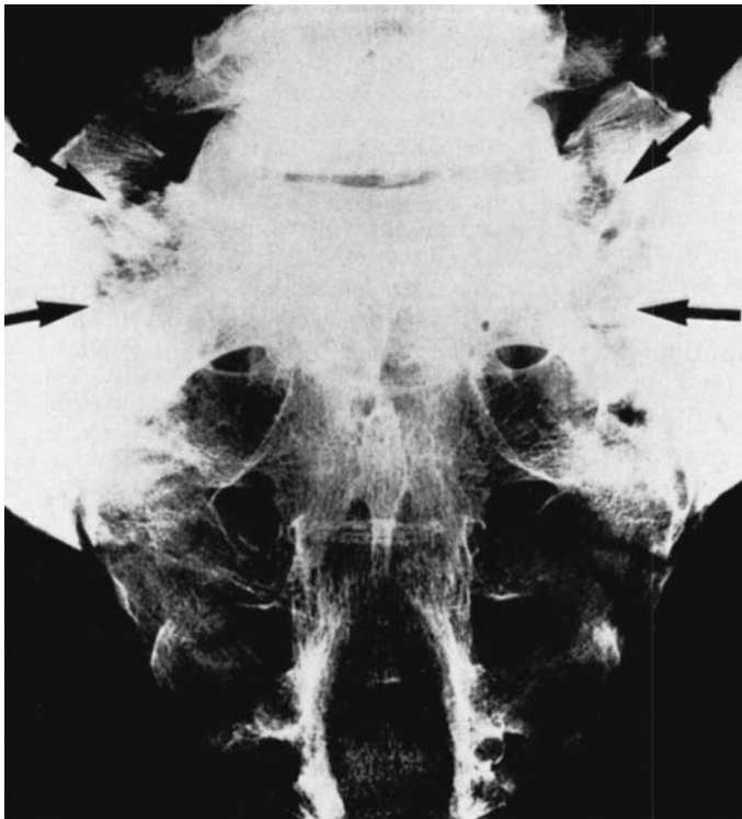
Figure 5. Radiograms of specimens showing fracture localizations. The initial fractures are indicated by arrows. a. Unresected specimen.
