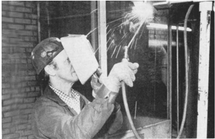
Figure 1. The working posture investigated. Overhead welding involves shoulder flexion and abduction.
