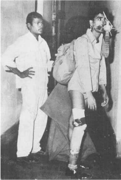
Figure 1. A below-knee amputee fitted with a PTB prosthesis and performing the graded load carrying test.
