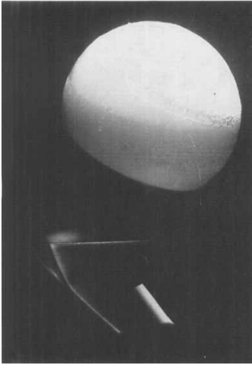
Figure 3. Circular lines of wear on the polyethylene cup of a prosthesis removed after 1 year.
