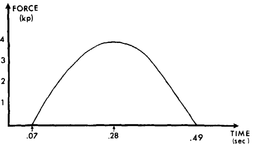
Figure 3. The dome shaped curve represents the force input into the right leg with each impulse load. This impulse load occurred 56 times per minute for 1 hour daily. The rapid rise and fall of the force input was selected to simulate joint loads which occur clinically.
