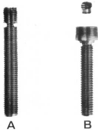
Figure 1. A. Chamber type A for implantation in the rabbit tibia. Chamber length 28 mm, outer diameter 4 mm. B. Chamber type B for implantation in the rabbit tibia. Chamber length 25 mm, outer diameter of the lower part 4 mm. This chamber type has a cover glass in a metal frame that is inserted into the chamber. The cover glass instead of the glass rod in type A permits the use of high resolution objectives.
