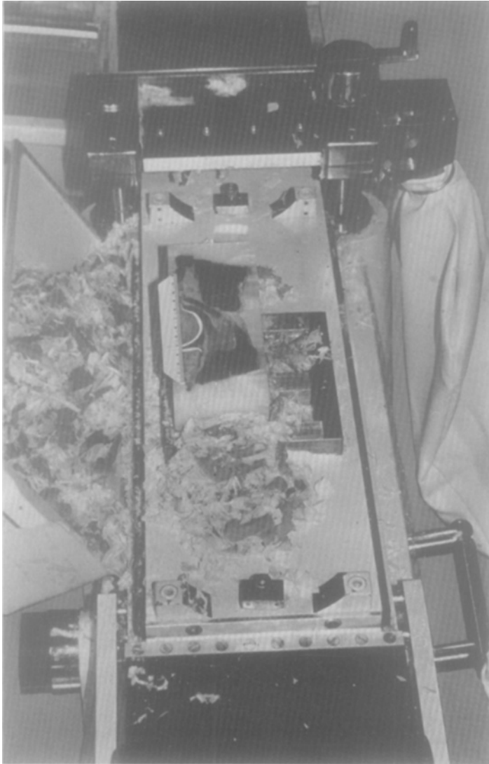
Figure 11. Serial cryosectioning with a heavy duty cryomicrotome built into a cryostat (LKB 2250 PMW). A human knee joint specimen with a communicating popliteal bursa is sectioned in the sagittal plane at -20^{\circ}\text{C} . The block is mounted on the horizontally moving sledge and the knife is fed downwards to cut sections 5–200 \mu\text{m} thick. The debris can be removed by a vacuum cleaner during automatic trimming.
