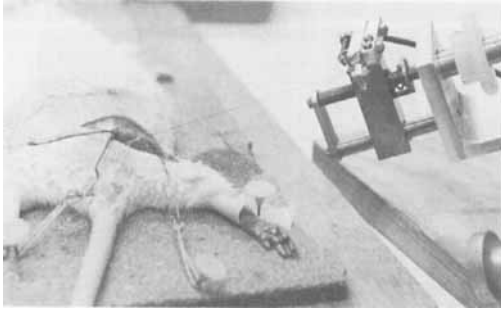
Figure 1. Arrangement of the apparatus for testing the properties of the proximal nerve section.
