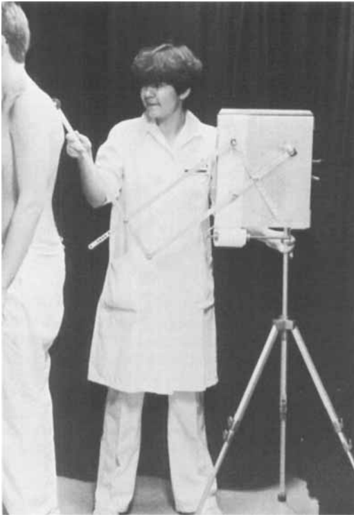
Figure 1. Spinal pantograph, when measuring kyphosis/lordosis.
