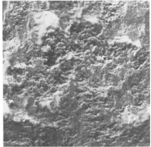
Figure 4. A slightly rough cut surface produced by the ultrasonic saw.
