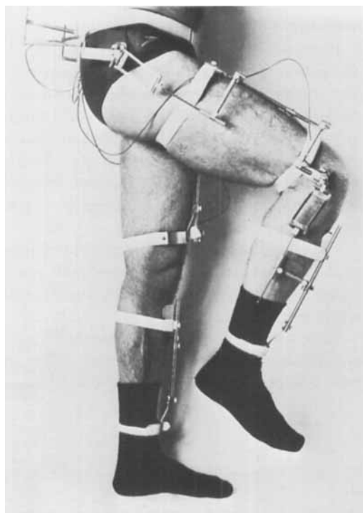
Figure 2. The electrogoniometric instrument applied on a subject.
