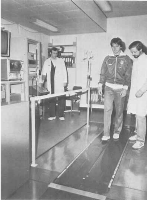
Figure 1. A person walking on the instrumented treadmill.
