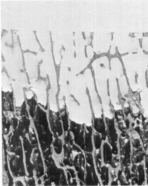
Figure 5. Longitudinal section of bone specimen following cement penetration. Trabeculae have been stained with silver nitrate solution to enhance contrast.
