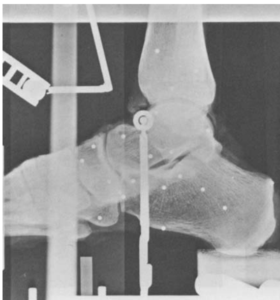
Fig. 2.11. Close-up of the central beam for the horizontal projection.
