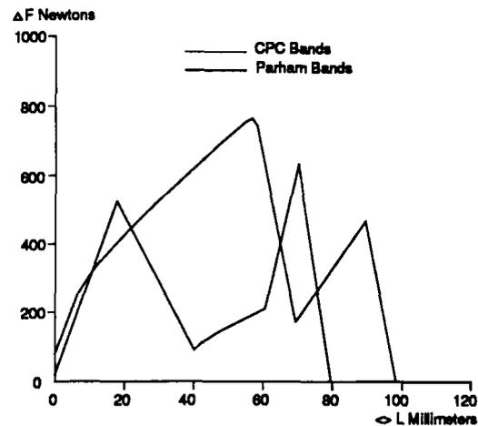
Figure 5. Comparative knot-slip resistance for CPC and Parham Bands.
