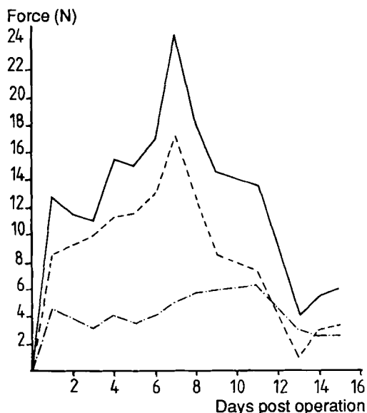
Figure 6. Force-time characteristics indicating fracture of the growth plate in one of the animals in Group B. The total force curve is obtained from the sum of the medial and lateral components of force measured from the fixator. Fracture is indicated at Day 7. — total force, --- medial component, - · - lateral component.
