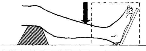
Figure 1. Posterior load of the tibia with the foot in the calibration cage. A posteriorly directed force was applied 20 cm proximal to the ankle by two weights attached to each end of a movable bar connected to the lower leg.
