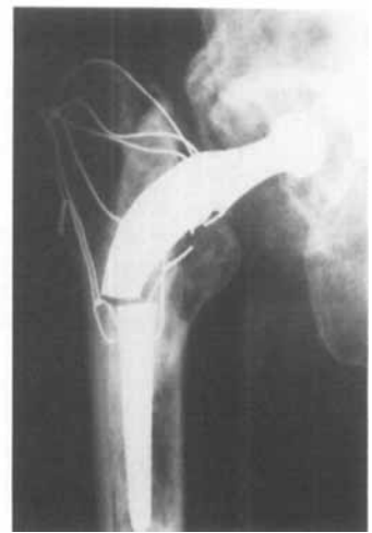
Another 5 months later, the femoral stem has broken.
