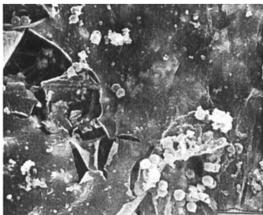
Figure 2. Scanning electron micrograph of tobramycin-impregnated PMMA. Bacterial microcolonies are seen on the biofilm or within it. Bar, 5 microns.
