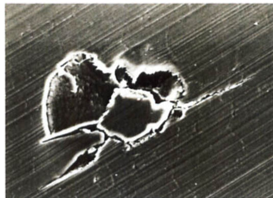
Figure 8. Scanning electron micrograph of fusion defect under the wear track showing initiation of cracks from the edges of the defect, x140. Duration 7 years.
