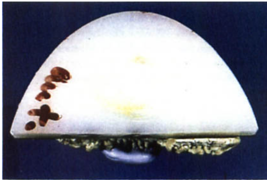
Figure 2. Photograph of retrieved St Georg tibial component (duration 7 years) showing break-up of the polyethylene surface due to delamination.
