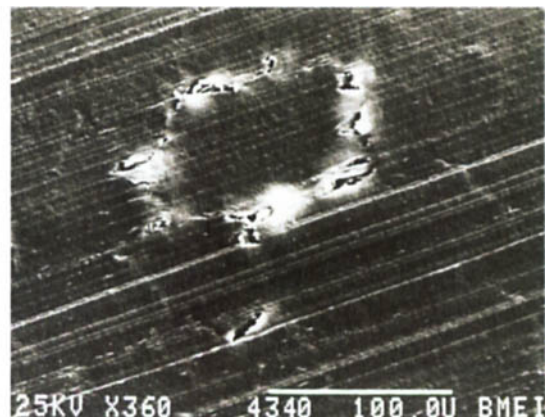
Figure 5. Scanning electron micrograph of fusion defect under non-worn region of polyethylene. The defect is partially bonded to the surrounding polyethylene, x400.
