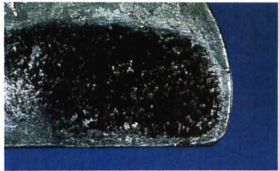
Figure 9. Photograph of retrieved Marmor tibial component. The component has been sputter-coated with a layer of gold to show clearly deformation of the wear track and the numerous pits, x5. Duration 7 years.
