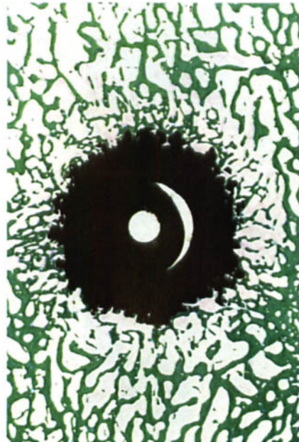
Figure 4 B. Cross section of a stable HA implant. Note the newly formed bone has filled the initial gap around the implant. Light microscopy, light green, basic fuchsin, ground section, \times 6 .
