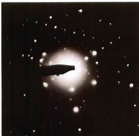
Figure 8. Diffraction pattern from a particle in the membrane around an HA-coated unstable implant. The electron wave is diffracted in the three-dimensional lattice of atoms, and the regular pattern indicates the crystal nature of the particle. Camera length: 950 mm.
