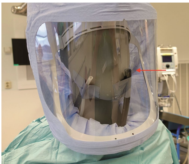
Figure 1. Test setup. The dummy with helmet, hood, and gown in the test setup. Arrow indicating particle counter inside helmet. (White probe is a passive pressure probe not used for tests reported in this paper.)
