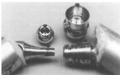
Figure 3. Conical contact surfaces of modular stainless steel femoral components corroded considerably during the tests (arrows). Thackray's head and Elite stem on the left, and Protek's head and Müller stem on the right. Stems are in their holders.
