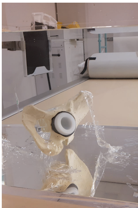
Figure 2. Sawbone of the hemipelvis placed in the Perspex box filled with 24.8 cm vertical water column.
