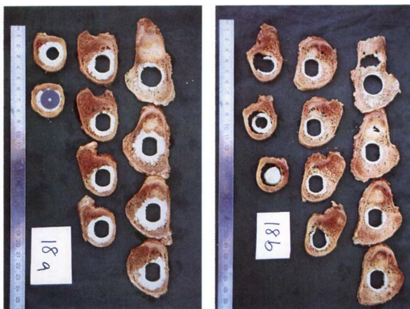
Figure 2. Cross-sections of femora after implantation, using cement-canal injection technique (left) at a pressure of 1.5 bar and control specimen (right). There are visible voids in cementation of the control femur, whereas no voids are seen in the femur with cement-canal technique.
