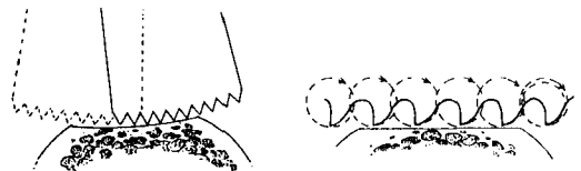
Figure 1. The oscillating saw mechanism (left) and the semirotating saw mechanism (right).
