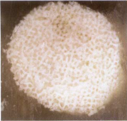
Macrophotography, 12 weeks. Only superficial attachment to host bone, no penetration inside the material. \times 10 .
