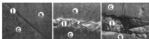
Figure 1.2. C indicates cement, S the prosthetic stem, and I the interface.
