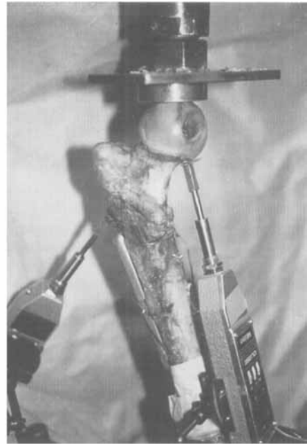
Figure 2. Intact femur in loading cell held in 25° of adduction in the coronal plane to simulate loading of a one-legged stance. One linear strain gauge and two displacement gauges are affixed as described in the text.
