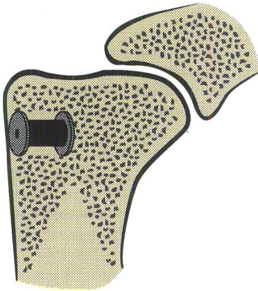
Figure 6. The unloaded implant is centralized in the drilled canal in the proximal humerus surrounded by a 2 mm gap. The deep part of the implant is fixed by the footplate in press-fit. A titanium washer centralizes the implant superficially.
