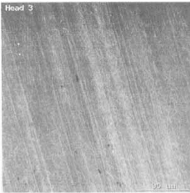
Figure 4. SEM from articulating surface of head 3.
