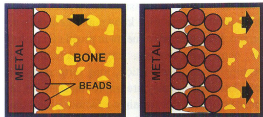
Figure 2. A multilayer of beads gives resistance to both shear and tensile loads.
