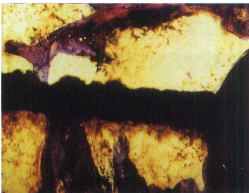
Figure 22. Hydroxyapatite coated cast mesh component at 2 years—bone ingrowth within the coating.
