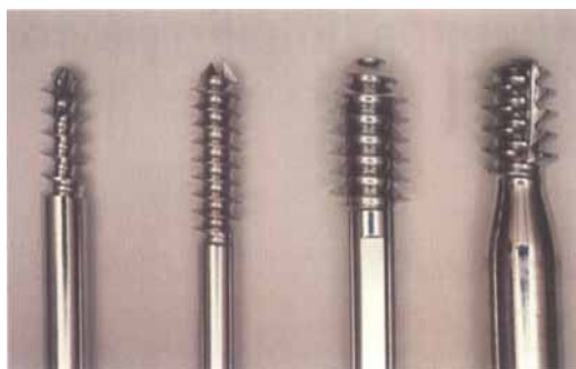
Figure 1. The 4 tested screws (from left to right): Gamma Nail, Dynamic Hip Screw, Uppsala Hip Screw, Ullevaal Hip Screw.
