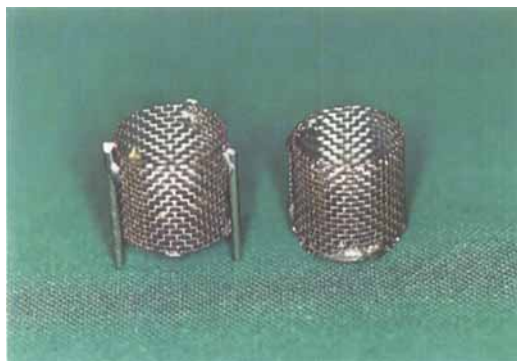
Figure 1. Wire-mesh cylinders were made of stainless steel. The wire-mesh cylinder used on the agar surface (left) had three small pins to maintain a fixed position on the agar. Antibiotic-impregnated bone was compressed into the cylinders.
