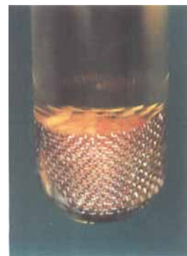
Figure 3. The antibiotics were eluted in Mueller Hinton broth at 37^{\circ}\text{C} by daily transfer of the cylinders into 5 mL of broth. The release of antibiotics into the broth was determined with a bioassay, using S. aureus ATCC 25923 as an inoculum.
