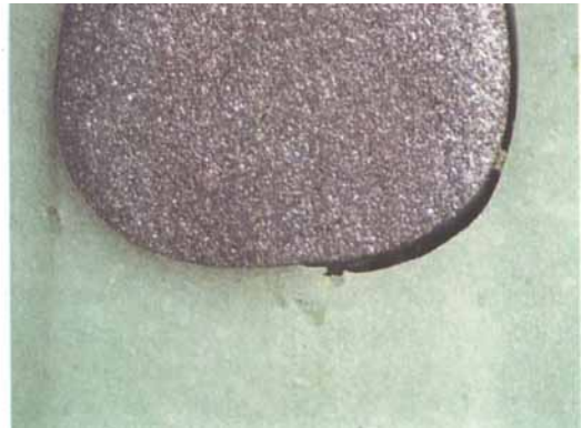
b. The close-up shows a gap with a sharp edge at the cement-stem interface.
